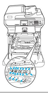
6 The jammed paper may be pulled out with the toner cartridge and drum unit assembly, or this may release the paper so you can pull it out of the paper tray opening.
